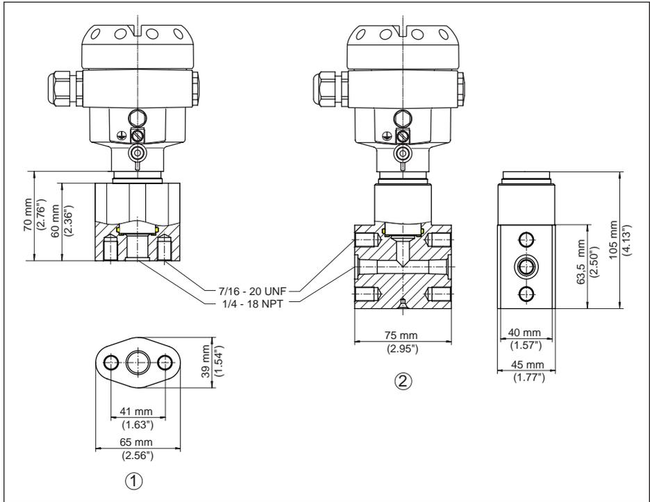
Fig. 45: CPT-2x, conexão conforme IEC 61518
