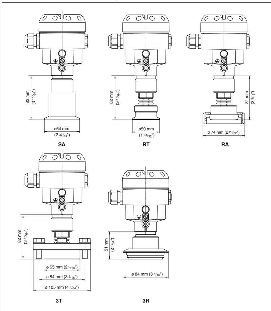
Figura 29: IPT-1\* Vers. 3.0, SA = Tri-Clamp 2", RA = attacco rapido filettato DN 40/PN 40 secondo DIN 11851, RT = Tri-Clamp 1½", 3T = DRD, 3R = Varivent Form F
