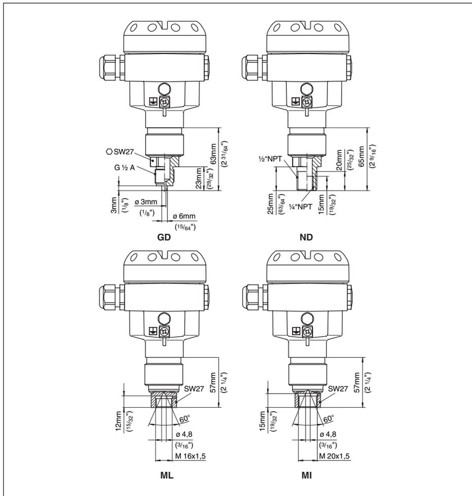
Figura 27: IPT-1\* Vers. 3.0 GD = G 1/2 EN 837, ND = 1/2 NPT, ML = M 16 x 1,5 interno, MI = M 20 x 1,5 interno
