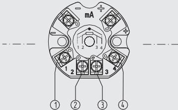
Identical dual sensors are supported for all sensor models, i. e. dual sensor combinations as for example Pt100/Pt100 or thermocouple type K/ type K are possible.
